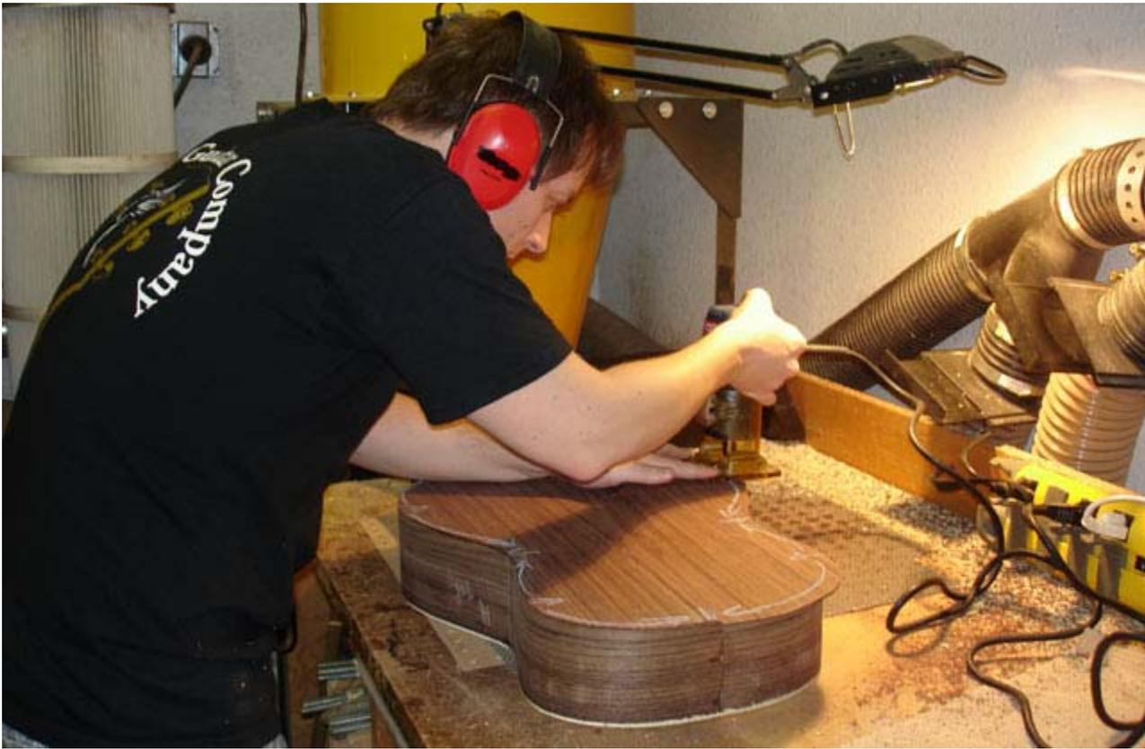
After the drying was complete I used a router to remove the excess overhang wood on both the top and back exposing what was now a “box” in its basic, final shape. The structural go-bars were then removed from the box by snapping them to fit through the sound hole. In a proud moment I tapped on the guitar to hear it resonate for the first time. I could feel the vibration of the sander across the room coming through the box too...a proud moment!
