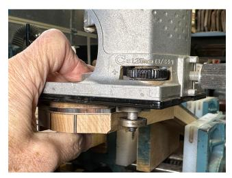
You can see how the router will ride along the headstock—on top of the MDF spacer. The cutter will cut a .090" cut into the edge of the headstock, and the bearing is riding on the headstock edge. Note that the cut will be just above the maple veneer at the edge of the headstock.
