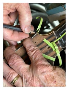
I will put a piece in place, and mark the angle with a pencil. Then I'll use my disk sander to sand the angle onto the binding piece—trying to leave it a little long—then, gradually take the piece down to final size. As I get two pieces together, I'll tape them down, and move on the the next corner.
