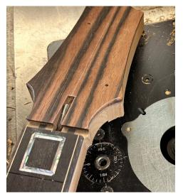
there is plenty of room for a cutter with a bearing to easily ride along the sides of the headstock. We're going to put a binding layer of about .066, with a purfling layer of about .022, to give a total of about .88 for the binding + purfling cut. One thing to note: the headstock veneer consists of three layers: The top-a thick (nearly 1/8 thick piece of macassar ebony, the middle, a 022" thick veneer of maple, and at the bottom, a .022" thick veneer of walnut.
