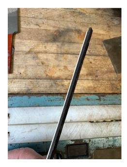
Here is the sandwich all glued up. I put glue between the layers, then clamped them together in a vise for about 30 minutes.
