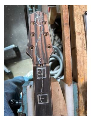
Here it is—with holes cut for the tuning machines, and a little inlay work done. Next, finishing...
