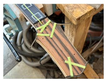
Here are the first pieces bent to the shape of the areas we want to cover. Next, we'll bend the longer pieces, and start to miter the corners.
