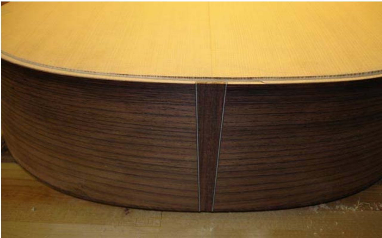
End graft complete and reading for purfling and binding
