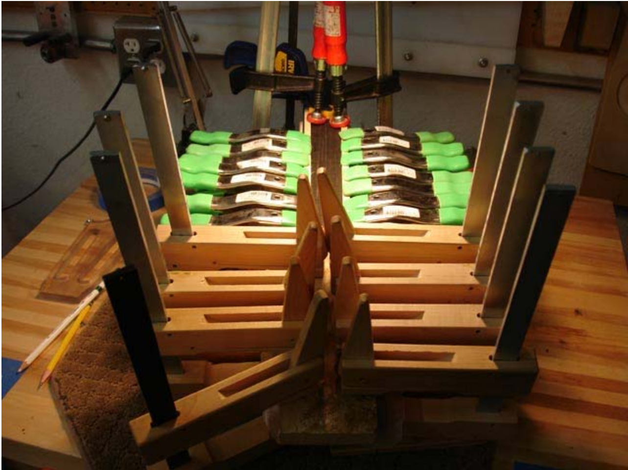
Fingerboard clamped to the neck
