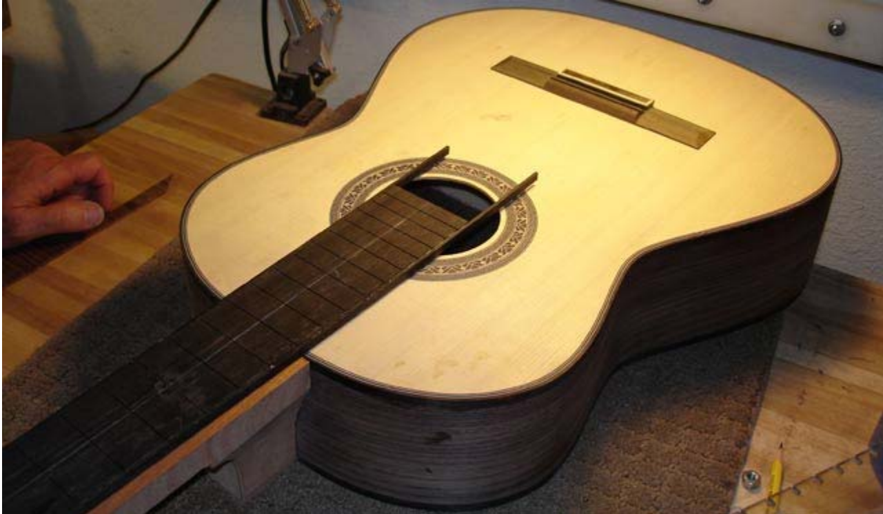
The guitar in its first semi-built state (with the fingerboard still extending into the soundhole)
