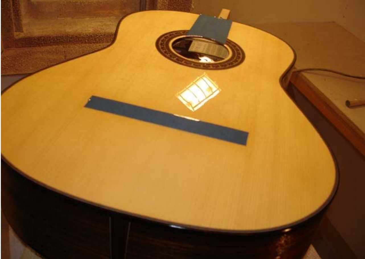
Clear coat drying
