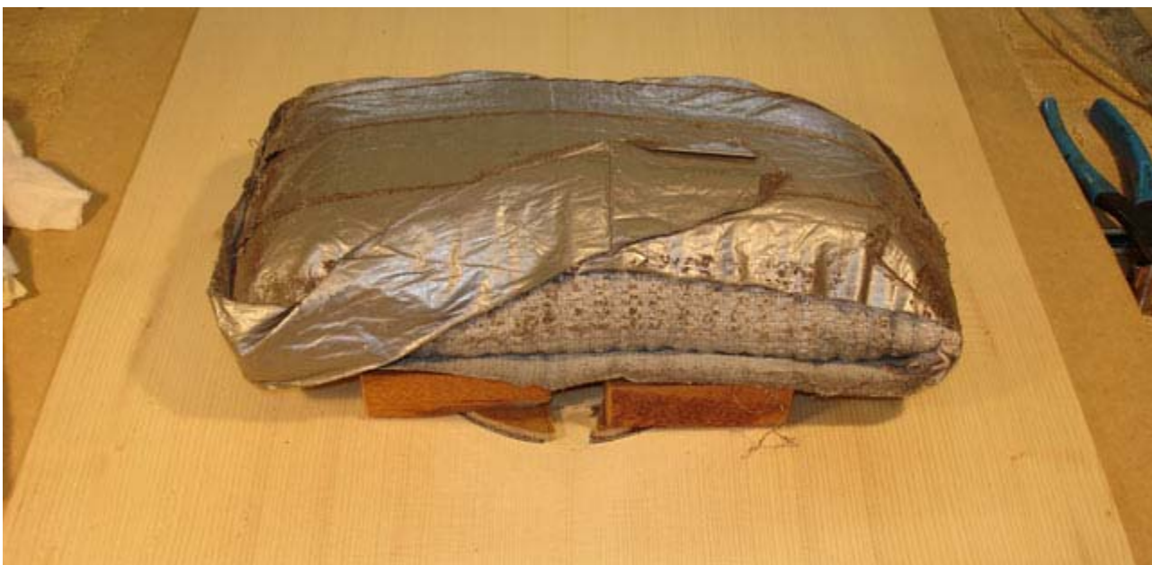
25lb. weight holds the rosette in place on the raw top.
