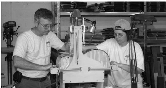
In photo 2, Mark can be seen scraping his top. Both the top and back on this guitar are made from pre-molded sitka spruce and flame maple, respectively. They are not laminates. We have found guitars made from this pre-molded material have several advantages: They are very strong, since the arch is not carved, so there is no runout from carving. The process of building is simplified, without having to completely carve the tops and
