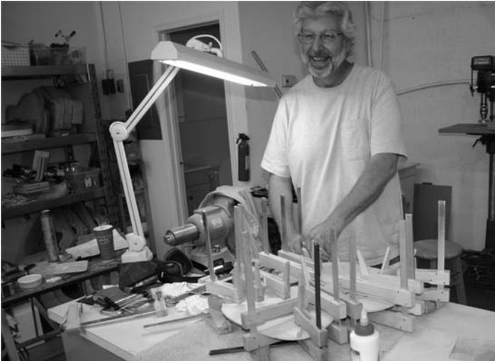
In photo 7, Mark gets the kerf glued onto the sides. He's nearly ready to glue on the top and back.
