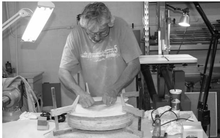
In Photo 3, Mark is preparing the braces for his top. He will be using x-braces. He is making guides using cam clamps, to help hold the braces in place, while he sands the profile on the bottom of the braces to match the inner curvature of the inside of the top.
